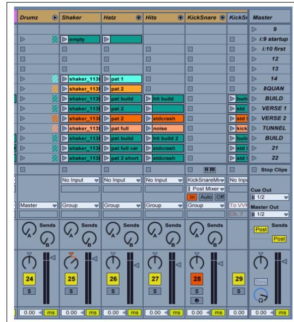
Figure 2. An example of a clip matrix in Ableton Live. The small play buttons are used to launch either clips or scenes and the column to the far-right represents scenes.
